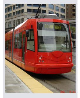
**Modern Streetcar** uses steel-tracked fixed guideways and electric-powered trains often electrified by an overhead wire. Modern streetcar typically operates in a lane with vehicles to fit easily into urban settings. Off-board ticketing, low floor vehicles, and multiple doors allow for faster boarding. Service operates as a single train and stations are spaced close together, typically every 1/4 mile.
