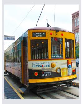
**Heritage Streetcar** uses steel-tracked fixed guideways and electric-powered vehicles electrified by an overhead wire. Vehicles are typically restored from or replicas of early 1900s vehicles. Service is often characterized as an urban circulator and consists of a single car or double car train operating on a city street. The track can run in its own lane or in a lane with vehicles.
