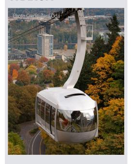
**Aerial Cable Transit** consists of passenger cabins suspended on cables. The fixed cables provide support for the cabins while an electric motor moves the cable. This form of transit is not a continuous corridor but instead is limited to the footprint of the cable support poles and station areas. Alignments are linear or straight with direction changes occurring at stations and/or special angle mechanisms.
