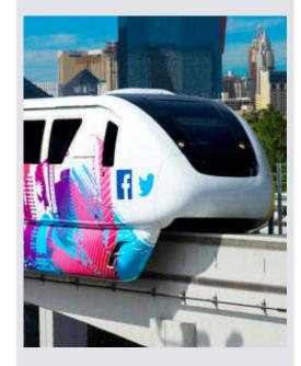
**Elevated Rail** is powered by electricity that runs through a rail below or above the vehicle. The electric rail requires it to operate exclusive from other vehicles and elevated above the street on a viaduct or other structure to protect riders from the electrical current. The technology has a larger carrying capacity than light rail and modern streetcar. Off-board ticketing, low floor vehicles, and multiple doors allow for faster boarding.
