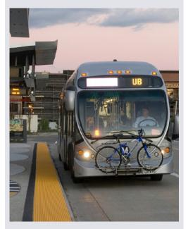
**Bus Rapid Transit** has specialized design, branding, services, and infrastructure that improve quality of service and reduce delay. Vehicles may be given priority at intersections. Off-board ticketing, low floor vehicles, and multiple doors allow for faster boarding. This service aims to combine the capacity and speed of rail with the flexibility, lower cost, and simplicity of a bus.
