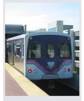
**Heavy Rail** is powered by electricity that runs through a rail below the vehicle. The electric rail requires it to operate exclusive from other vehicles to protect riders from the electrical current. Heavy rail operates in 2 to 12 car trains and has a larger carrying capacity than light rail and modern streetcar. Off-board ticketing, low floor vehicles, and multiple doors allow for faster boarding.
