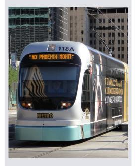
**Light Rail** uses steel-tracked fixed guideways and electric-powered trains often electrified by an overhead wire. Vehicles operate in their own lane and can operate as a single train or as multiple vehicles coupled together. Off-board ticketing, low floor vehicles, and multiple doors allow for faster boarding. The term "light rail" was coined to convey the vehicle's design, "..for light loads and fast movement."
