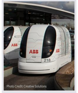
**Autonomous solutions** are fully automated forms of transit with rubber-tire vehicles operating along a guideway. The most common application in the U.S. is at airports, such as Tampa International. These systems span a variety of designs, from subway-like advanced rapid transit (ART) systems to smaller car-like vehicles known as group rapid transit (GRT) with vehicles sized for around 20 passengers.
