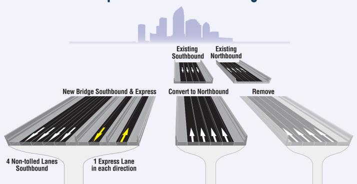
FDOT is replacing the existing northbound bridge (the one closest to the Gandy Bridge) due to its age. Once the new bridge opens, it will carry the four non-tolled lanes of southbound traffic like what is currently available, and also one express lane in each direction. The existing southbound bridge will be converted to northbound traffic.
